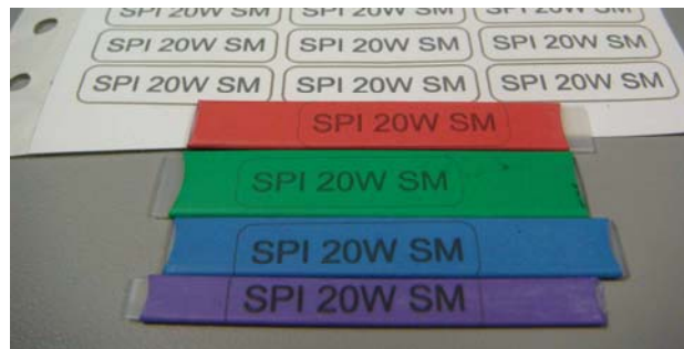
Image 9 Marking and cutting outline of labels in heat shrink material samples courtesy of Thinklaser
