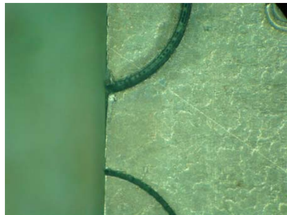
Image 2 Arcs cut showing effect of increased kerf width resulting from beam wobble (top) vs no wobble (bottom)
