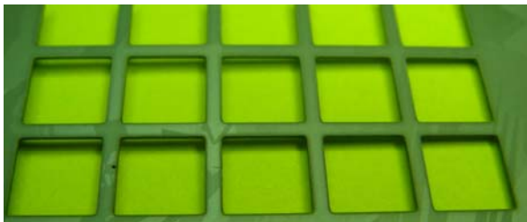
Image 7 Squares cut from 200µm thick polycrystalline silicon sample courtesy of University of Lisbon, Faculty of Sciences
