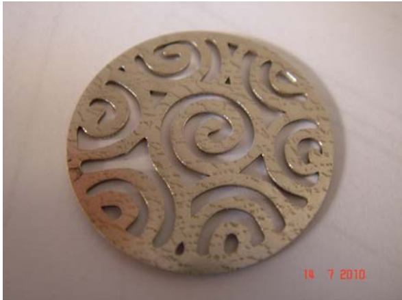
Image 6 Silver disc 0.55mm thick cut with 20W in 13minutes image courtesy of Orotig srl
